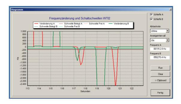
The displayed diagram indicates the actual frequency changes and switching threshold of the connected loops for a specified time period. Sampling rates and interval can be set individually.
