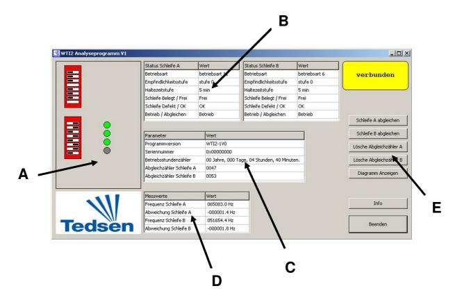
A: Actual settings of the DIP-switches and the LED status of the connected WTI2
